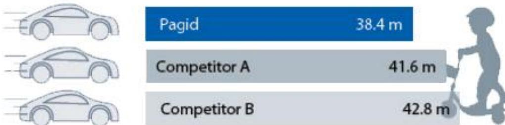
Braking distance (cold) from 100 km/h under maximum deceleration
