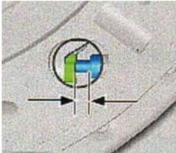
If the park brake shoe lever and park brake cable are not as shown, proceed to the next step (8)
